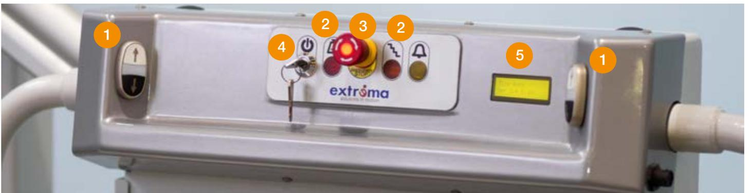
1. The **controls** for rise and descent are **easily reachable** by any user on every side of the instrument board.
